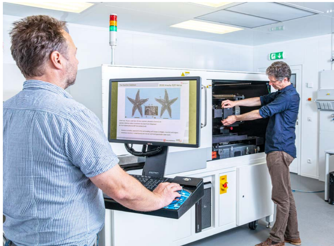
← The 3D X-ray microscope ZEISS Xradia 520 Versa at the MAPEX Core Facility. Photo: Matej Meza / University of Bremen
