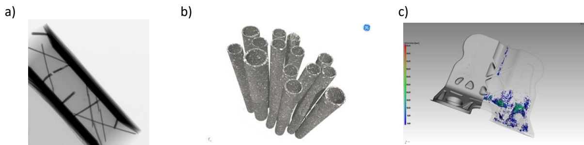
Fig. 2: a) X-ray image of a compression- and impact-loaded pin-reinforced sandwich structure; b) 3D view of bi-component fibers ( \varnothing ca. 200\ \mu\text{m} ); c) short fibre injection moulded T-bracket, 3D view and color-coded pore analysis.
