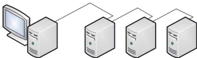
Abb. 1: EtherCAT-System - 1 Master + 3 Slaves
