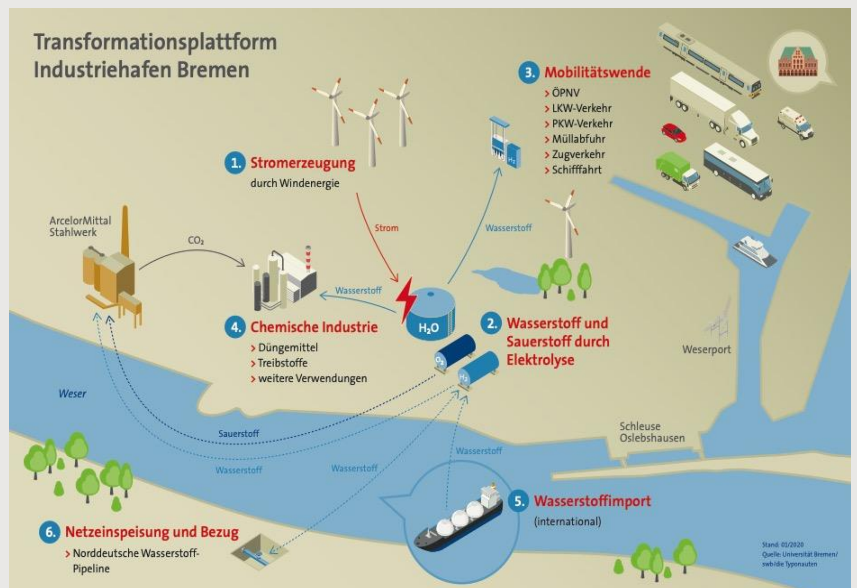
Figure 3: Schematic overview of the planned H2B transformation platform around the industrial port Bremen Source: adaptation of University Bremen swb / die Typonauten
