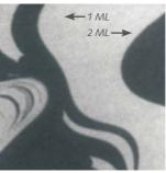
left image: single (bright) and bilayer (dark) graphene flakes on a SiC(0001) substrate (field of view: 3 µm).
