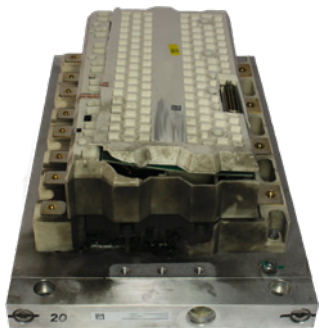
Fig. 2: Failed wind converter power electronics module. Numerous of these modules are build into a wind converter system.
